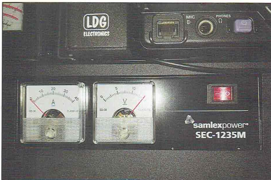
Photo B. The Samlex SEC-1235M power supply is available for rack-mounting as well as standalone operation.
